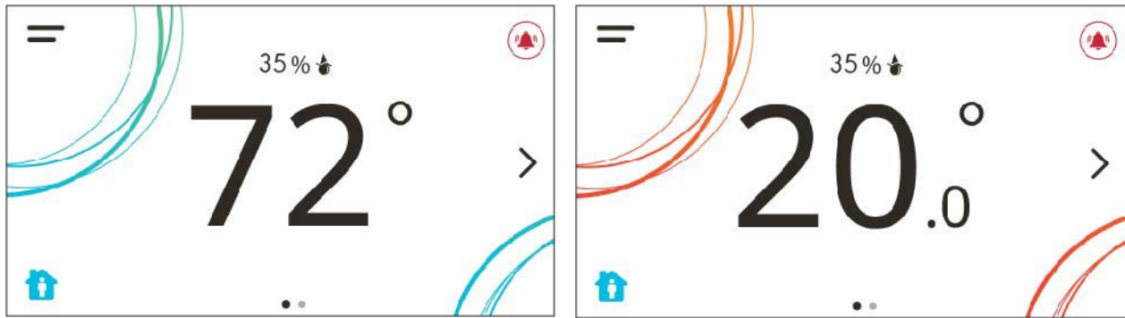
Figure 22: Thermostat controller home screen in cooling mode (left) and heating mode (right)
